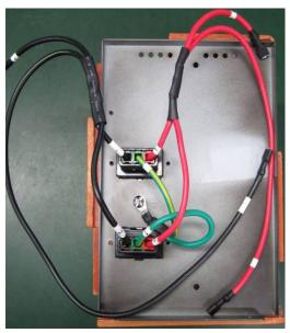
2. Please assemble the 6PCS batteries with black wire and place 6PCS batteries into the Battery Case as below.
