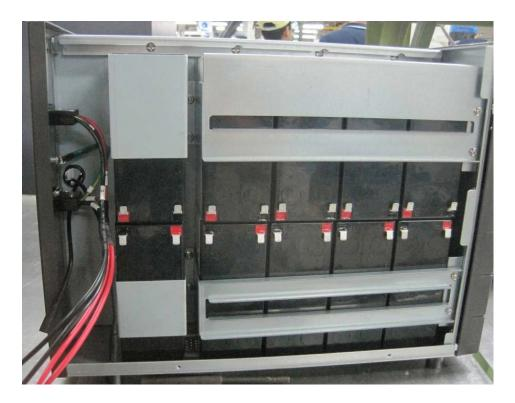
5. Please connect batteries on the left side with wires as below:
