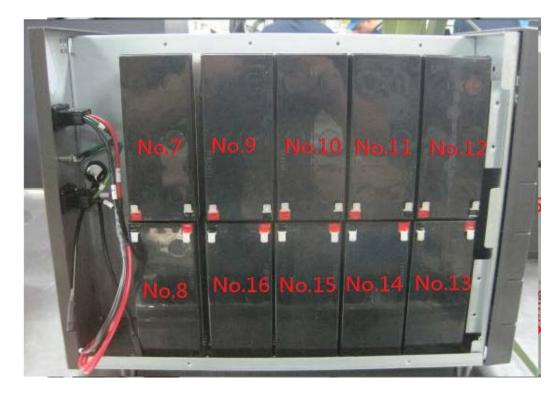
Pass through the cables 560mm & 370mm to the hole
