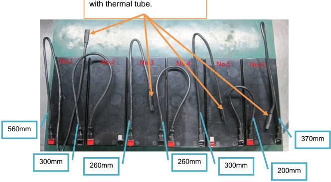
The connectors should insulate with thermal tube.
