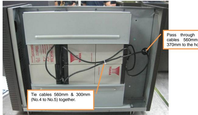
4. Please assemble 10pcs batteries into the Battery Case's left side and assemble with fixing plates as below.
